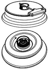
To ensure aerosol sealing the lid of an aerosol sealed angular rotor must be firmly closed. This is performed with the help of the supplied spanner that is inserted through the borehole in the rotary handle. If the rotary handle does not have a borehole then the lid must be firmly closed by turning in clockwise direction.
